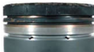
The leading North American brand low-ash NGEO left carbon deposits in the ring zone of this piston. Deposits that cause loss of power and increase engine wear.
