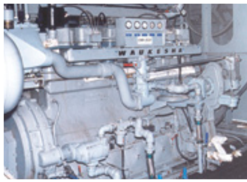
Petro-Canada’s SENTRON 470 was tested in this 810-horsepower Waukesha VHP F3521GSI engine.
